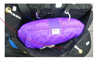
Check if the zipper puller offers risk to hook the line or cause malfunction of the rescue use
